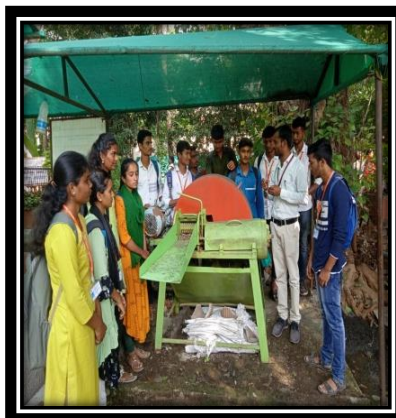
Vermicompost Shed Chaff cutter used for cutting leaves used in vermcomposting
